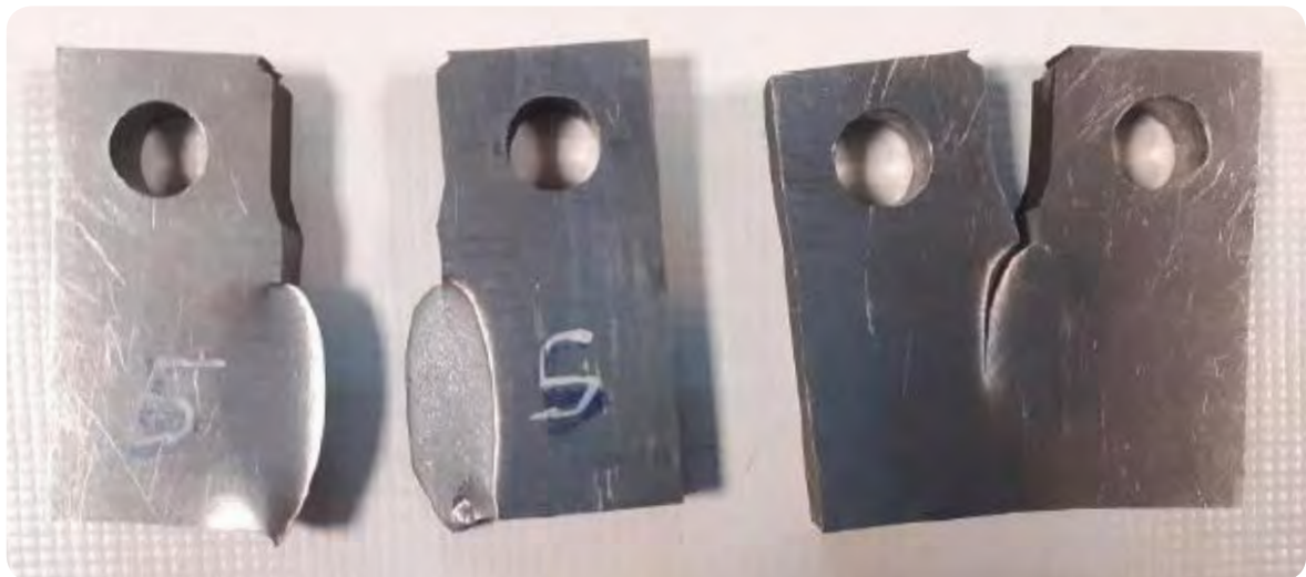
Fig. 5 – Broken fracture toughness test specimen
