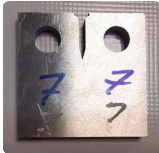
Fig. 4 – The fracture toughness test specimen
